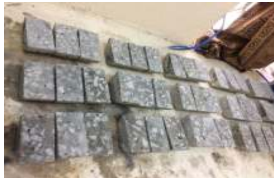
Fig 14: Chloride migration test
